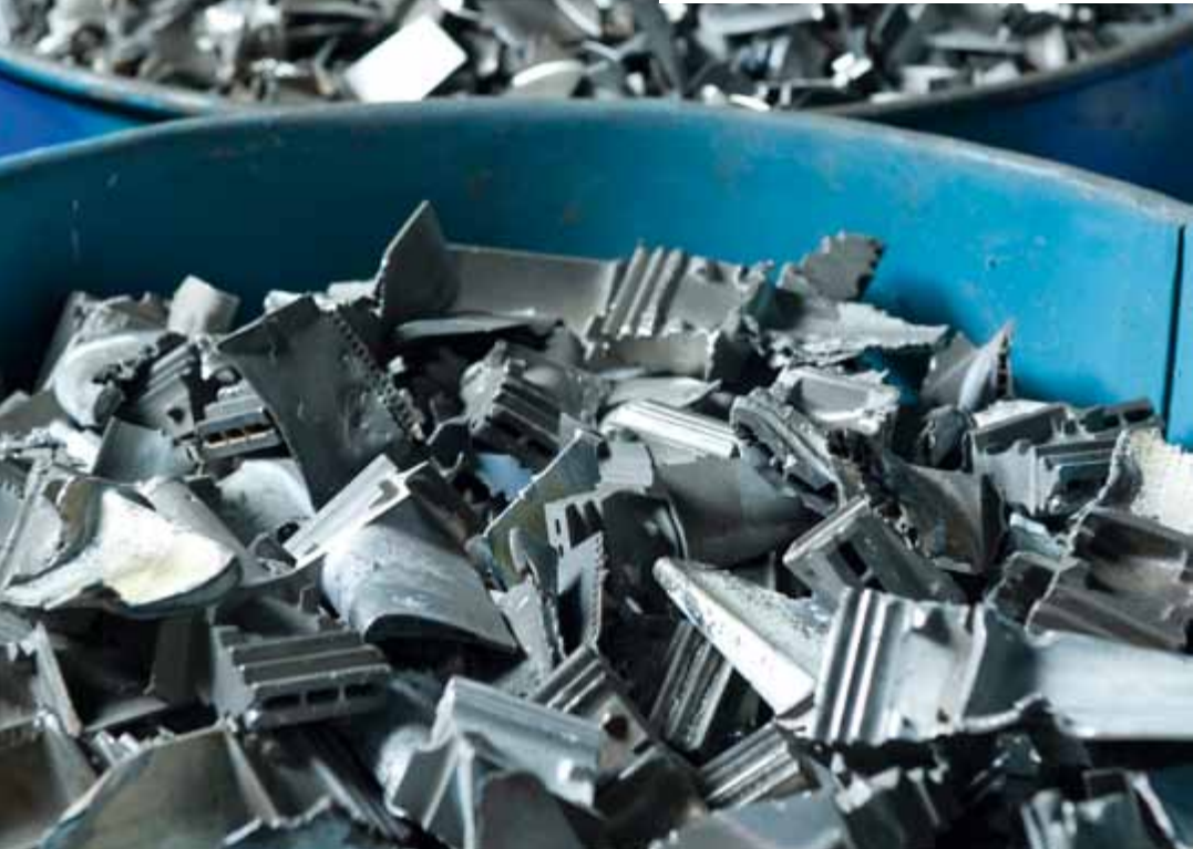
Duly mutilated turbine engine blades
