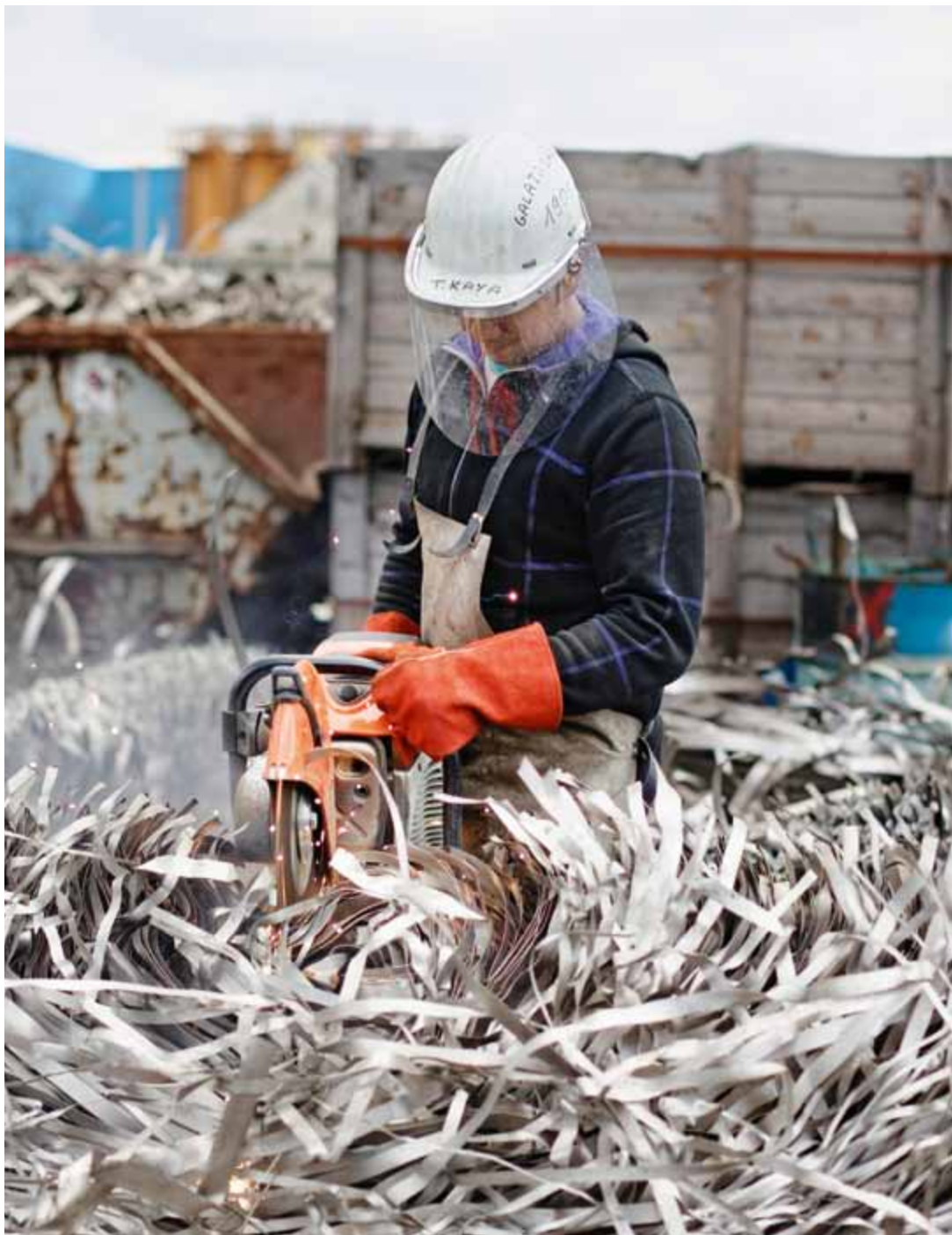
Metal bands being cut to size for further processing with a motorflex saw
